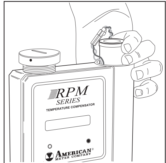
Fig. 15 Removal of the Battery
